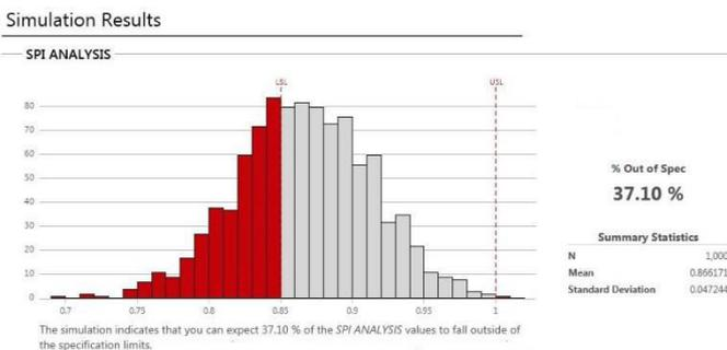
From the above two cases we can understand that the specification limit of 0.75 to 1, which will suitable for our project. So we can set a Schedule Performance Index (SPI) within this limit for better monitoring of the schedule of the project.
